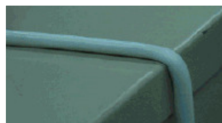
Fig.2 Cable with small bending radius provide flexible network deployment
