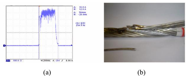
**Figure 3. Waveform (a) and sample (b) of OPGW-I after the first 250C lightning shot (three wires were broken)**
