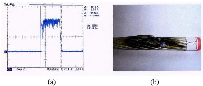
**Figure 2. Waveform (a) and sample (b) of OPGW-I after the second 200C lightning shot (two wires were broken)**
