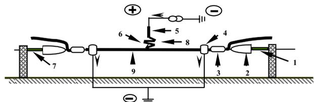
1. Turnbuckle, 2. Insulator, 3. Anchoring clamps, 4. Earthing connectors, 5. Electrode, 6. Metal fuse for ignition, 7. Tension meter, 8. Gap between electrode and cable surface, 9. Test sample
