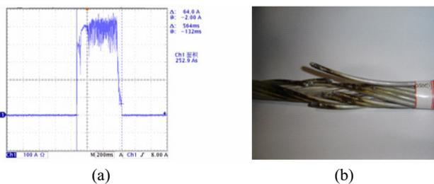
**Figure 5. Waveform (a) and sample (b) of OPGW-II after the first 250C lightning shot (four wires were broken)**
