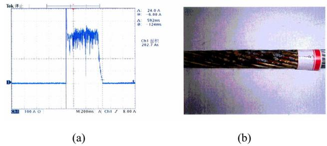
**Figure 6. Waveform (a) and sample (b) of OPGW-III after the fourth 200C lightning shot (no wires were broken)**
