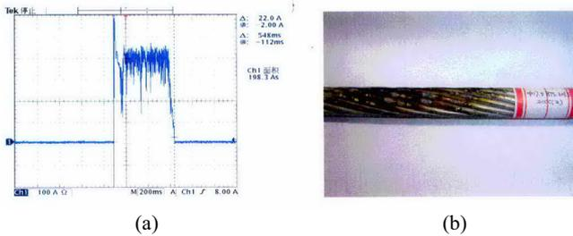
**Figure 4. Waveform (a) and sample (b) of OPGW-II after the second 200C lightning shot (no wires were broken)**
