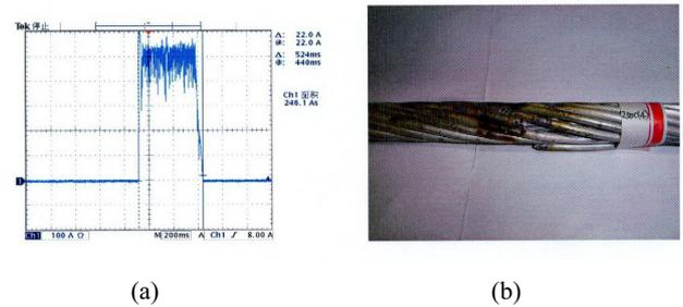
**Figure 7. Waveform (a) and sample (b) of OPGW-III after the fourth 250C lightning shot (one wire was broken)**
