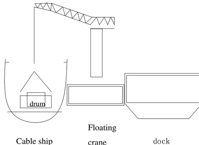
Schematic diagram of wholly hoisting cable conveying with basket
